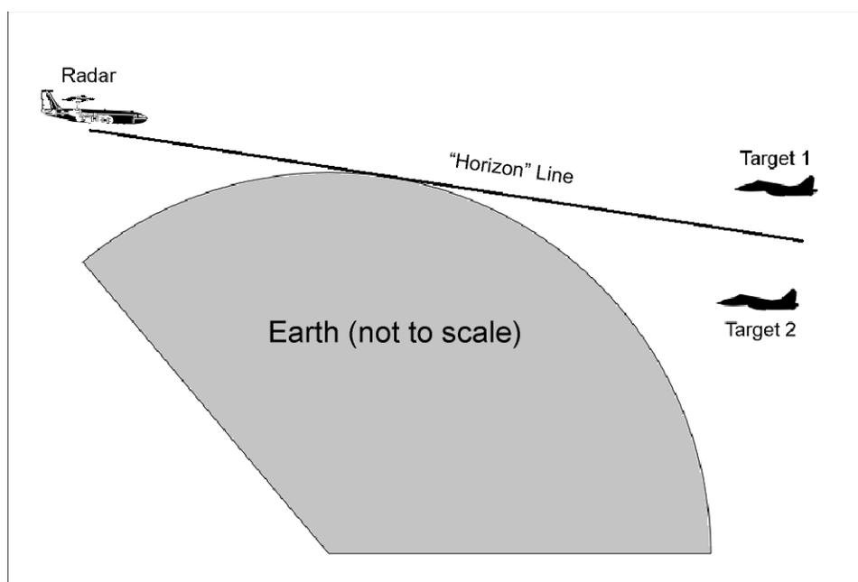
**Figure 388: The Earth's horizon blocks radar. Radars without OTH capabilities would only be able to detect Target 1. Those with OTH capability would be able to detect both. The horizon calculations include the radar and target heights above ground level (AGL).**
