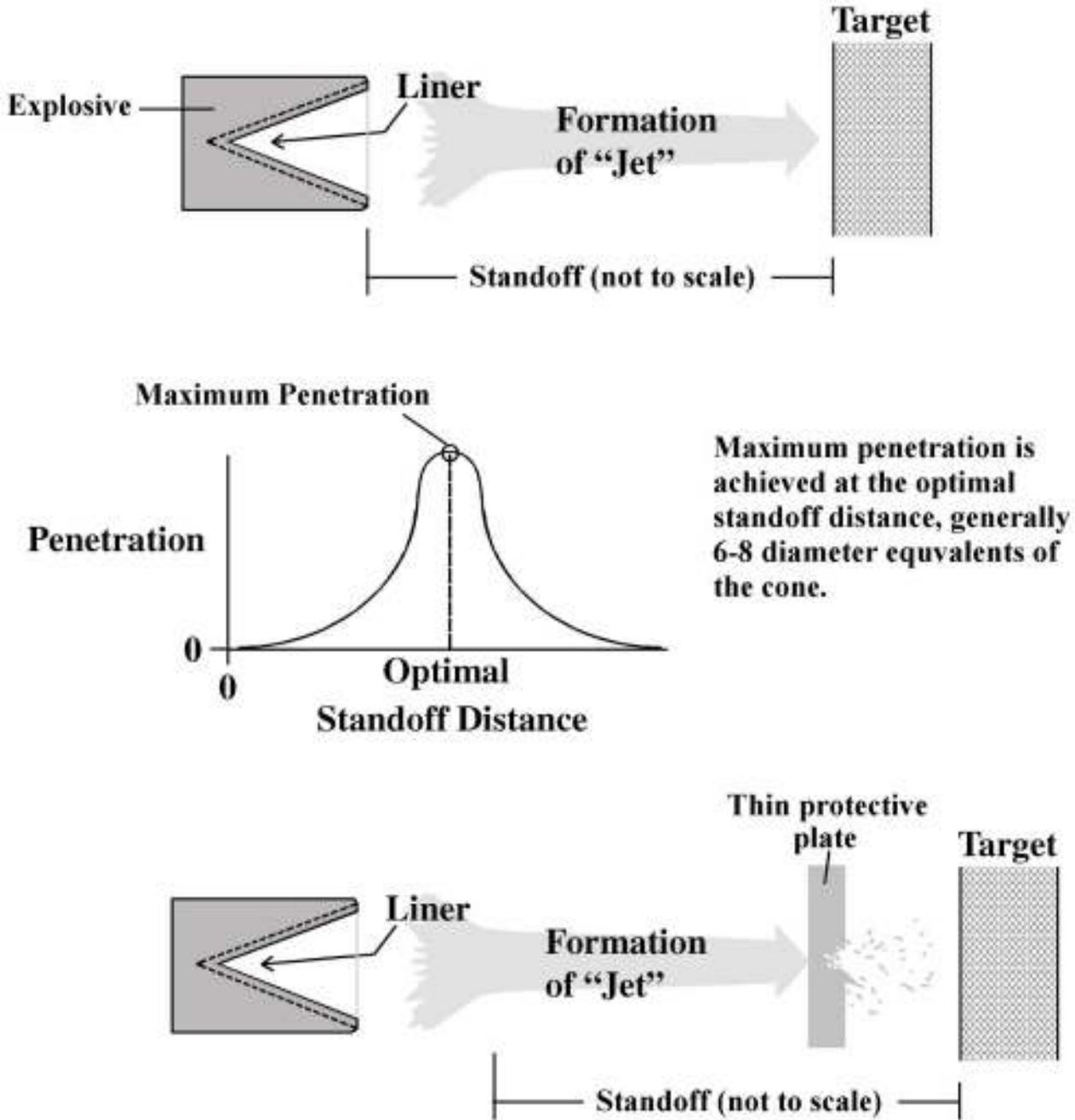
**Common countermeasure - thin protective plates cause premature detonation of the warhead outside the optimal standoff.**
