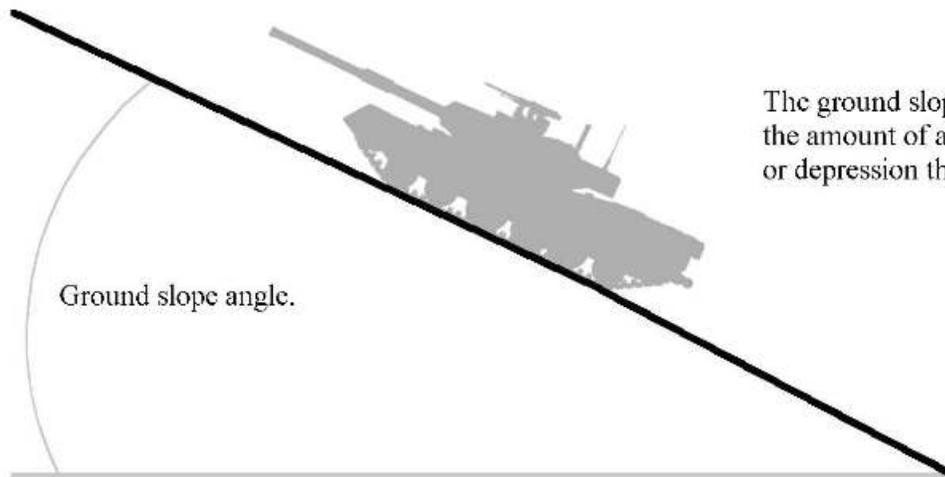
The ground slope (up or down) affects the amount of additional gun elevation or depression that is required.
