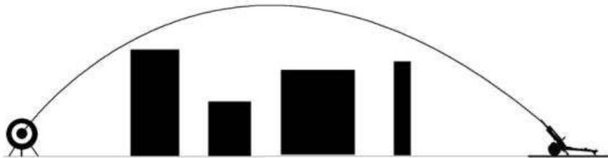
Ballistic (unpowered) flight paths must clear all obstacles. The firing angle must be within the gun/launcher capabilities.
