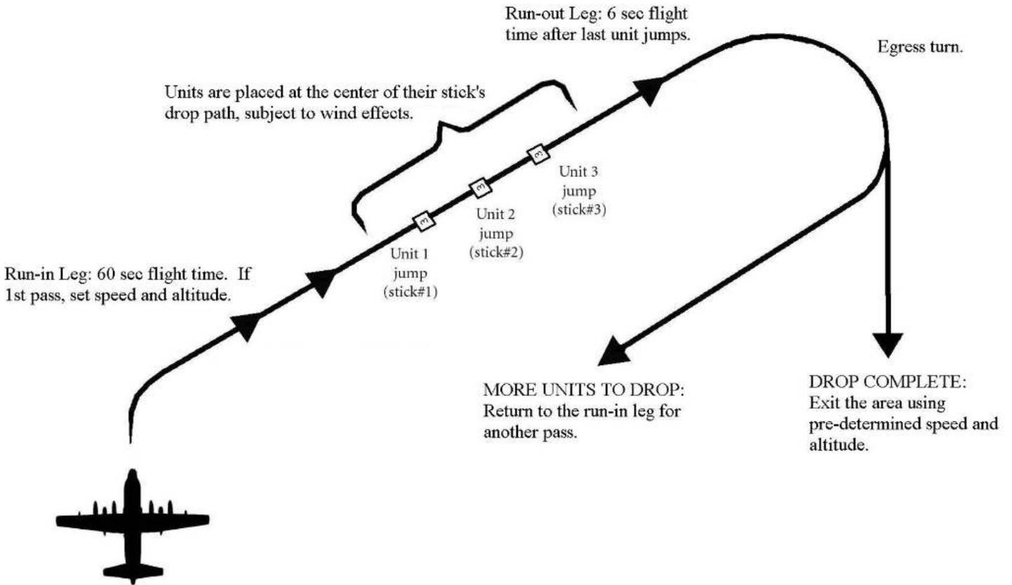
**Figure 395: The basic paradrop flight path and stick locations relative to the intended drop zone. Note the sticks belonging to unit 1 jump first, followed by the sticks from the other units, even if the sticks are on different aircraft or jump on different passes. The result is all of the jumpers from unit 1 will eventually land at the near end of the DZ, those from unit 2 in the middle, and those from unit 3 at the far end.**
