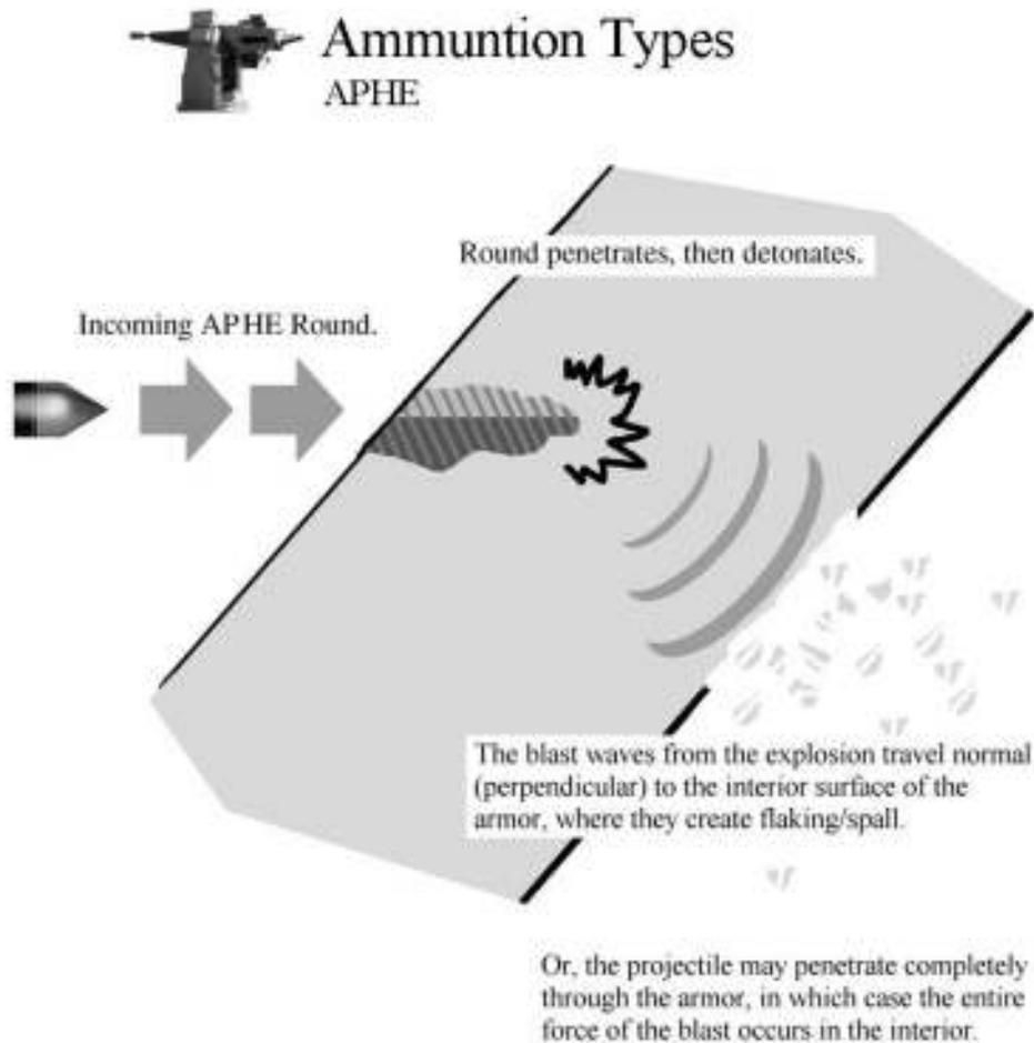
**Figure 360: APHE (Armor Piercing High Explosive) projectile fundamentals.**
