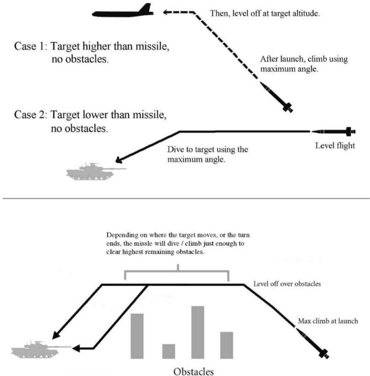
Figure 352: Powered In-flight units follow simple flight paths. If the in-flight munition is guided, the flight path is periodically adjusted to account for target movement.
